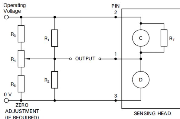
$$R_1 = R_2 = 500\Omega \text{ to } 10 \text{ k}\Omega$$
